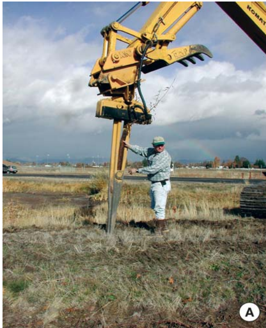
Figure 10.3.4.8. The expandable stinger is operated by placing a long container or hardwood cutting into the chamber (A). The arm of the excavator pushes the point of the stinger into the soil to the appropriate planting depth for the root system (B) and the beak opens, shattering the soil (if it is compacted) and creating a hole (C). The stinger is removed and the plant remains in place as soil collapses around the sides of the plug (D).
