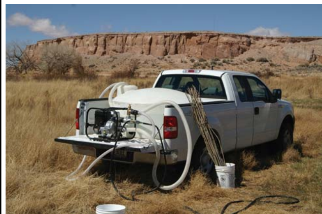
Figure 10.3.3.4. A 250-gallon water tank with pump can be installed in the bed of a pickup truck to supply water for Waterjet Stinger sticking.
