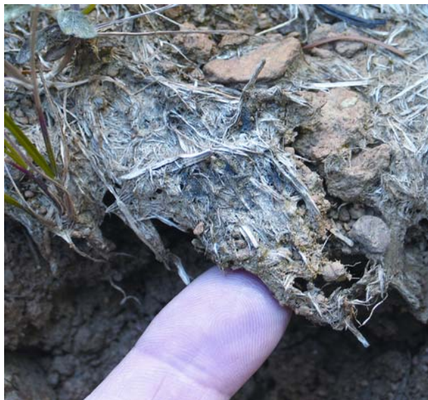
Figure 10.3.2.9. Hydraulic mulch with tackifiers remain effective for up to a year. This hydraulic mulch and tackifier slurry was applied nine months prior to this picture, and was still partially effective.
