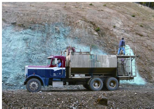
Figure 10.3.2.1. The hydraulic seeder is composed of a tank that holds and mixes a slurry, and a pump system that moves the slurry through a nozzle for application to the soil surface.
