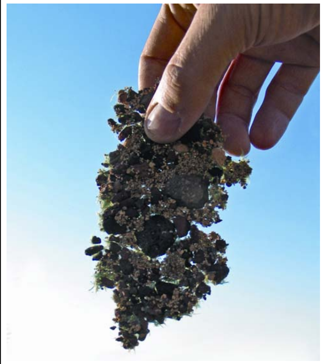
Figure 10.3.2.7. Hydraulic mulch applied at high rates and with specialized tackifiers will hold together as a sheet and is referred to as a “bonded fiber matrix,” or BMF. The application rate of wood fiber mulch in this picture was 3,000 lb/ac.
