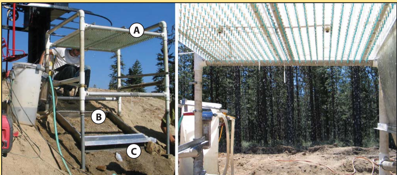
Figure 5.48 - A portable “drop-forming” rainfall simulator developed by scientists at University of California Davis (Grismer and Hogan 2004) delivers water droplets through hundreds of needles (A). Pressure is increased or decreased to simulate rainstorm events. Droplets hit the surface of soil within a plot frame (B) and runoff water is collected at the bottom of the frame (C) to measure runoff rates and sediment production.
