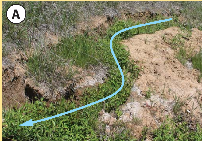
Figure 5.59 - Slumps are characterized by scarps, cracks, and benches. Water collects on the benches and in the cracks where it is transmitted into the slide mass, creating continued instability. Water can be removed through a series of hand-dug surface ditches. Using the cracks as guides for the location of ditches, they are filled in with soil and dug wide enough for a willow fascine (see 10.3.2.4 Live Fascines) to be placed in the bottom (A). Called “live pole drains” (Polster 1997), these structures not only quickly move surface water off the slide to more stable areas, but the willow cuttings in the fascines, encouraged by the presence of high soil moisture, grow into dense vegetation (B) that stabilize the slide through the deep rooting and dewatering.
